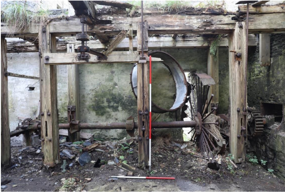
Figure 19: Remains of wheel and drive shaft
