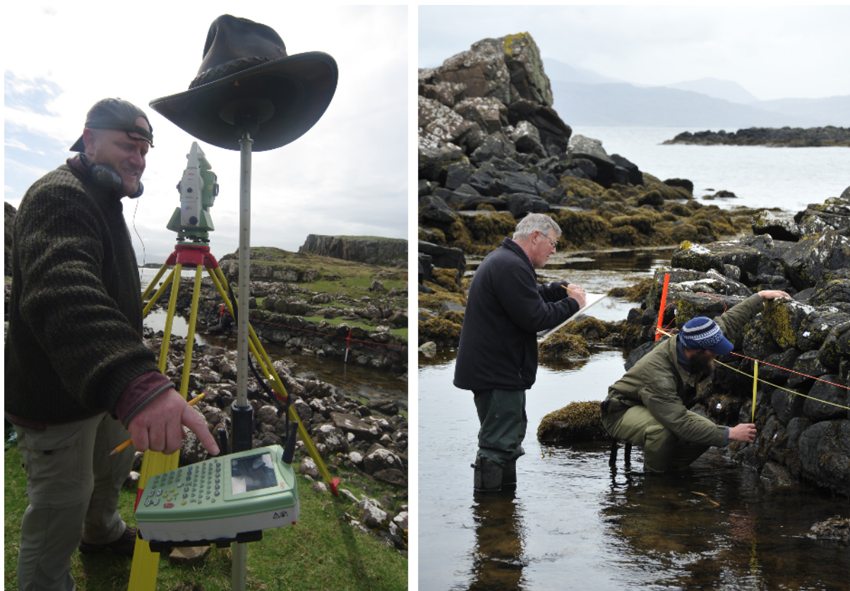
Figure 9. Left: reflectorless EDM survey. Right, setting out datums for PhotoModeler survey (Colin Martin; Edward Martin)
