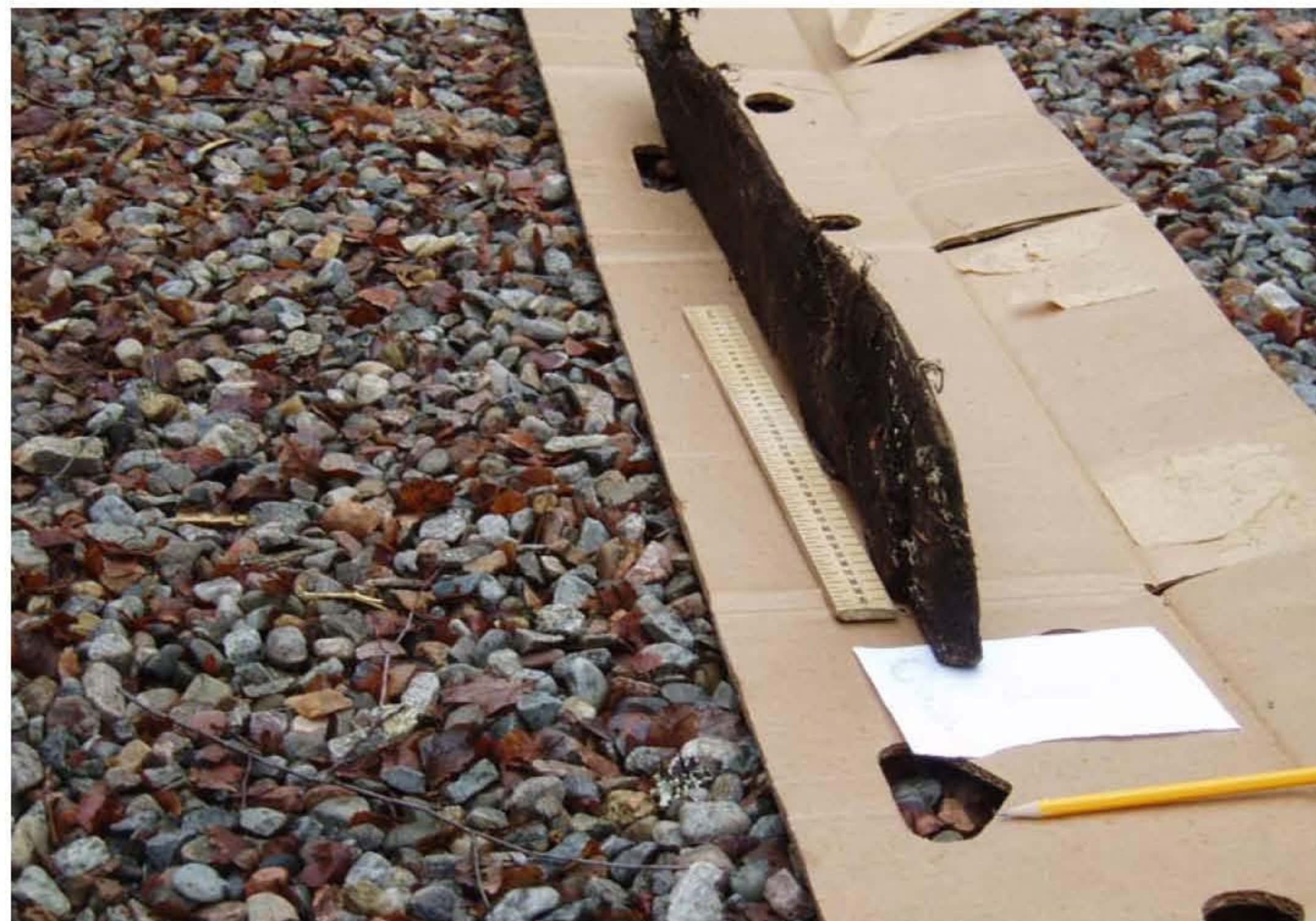
10 - plank 1 - resting on straight edge showing wedge profile
